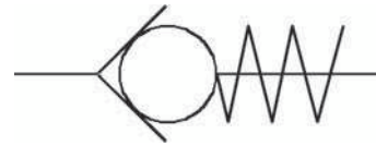
Rückschlagklappe federbelastet (Option) Spring-actuated swing check valve (optional)
