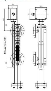
Clearance dimensions C [mm] with DIN V flange
