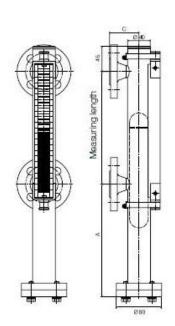
NBK-M... with roller-type display and magnetostrictive transmitter
